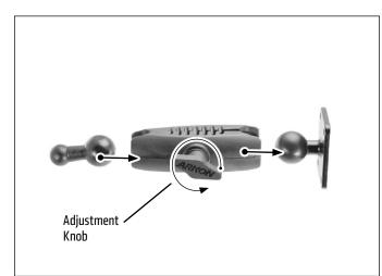
B Use appropriate screws (not included) to secure mount to mounting surface. Use anchors if necessary. Loosen adjustment knob, set to desired position, and retighten to set.
